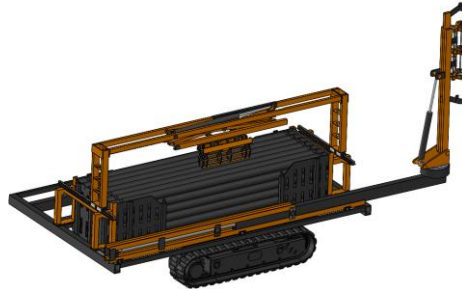
FIGURE 1 Proposed equipment for handling drill pipes.
