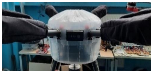
FIGURE 1 Preliminary demo PP cover mounted on INCAS UAV developed via vacuum thermoforming
