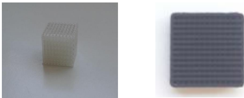
FIGURE 1 3D printed scaffolds made of (a) PLA, 500 \mu\text{m} square shaped pores and (b) PLA reinforced carbon nanoparticles, 500 \mu\text{m} square shaped pores
